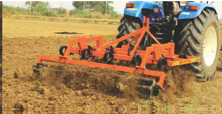
Double coil spring action tyne
