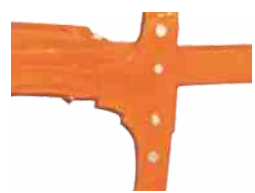
Boron steel tynes with overload protection
