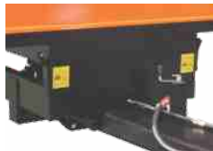
Detachable drawbar for increased loadability
