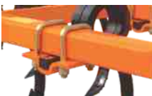
U clamp for attachment & adjustment of tyne
