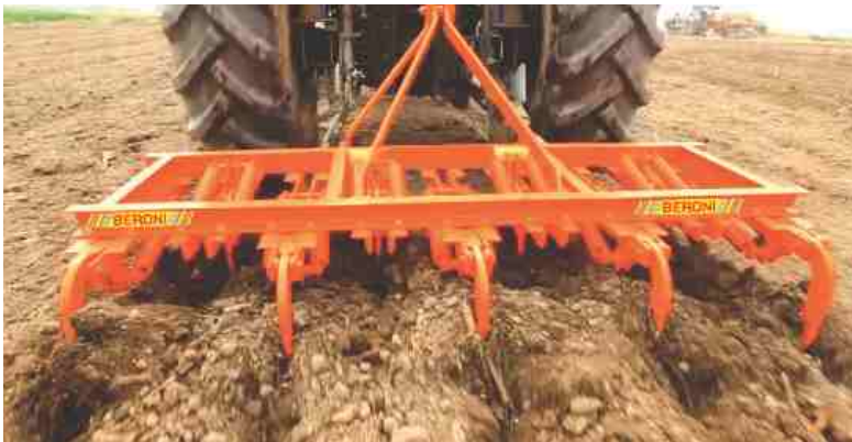
Spring having more capacity of absorbing shock
