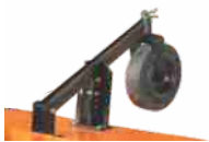
Tyre assembly for depth control
