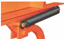
Spring having more capacity of absorbing shock
