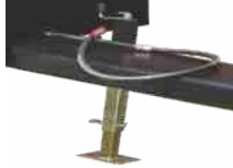
Vertical screw jack for easy parking
