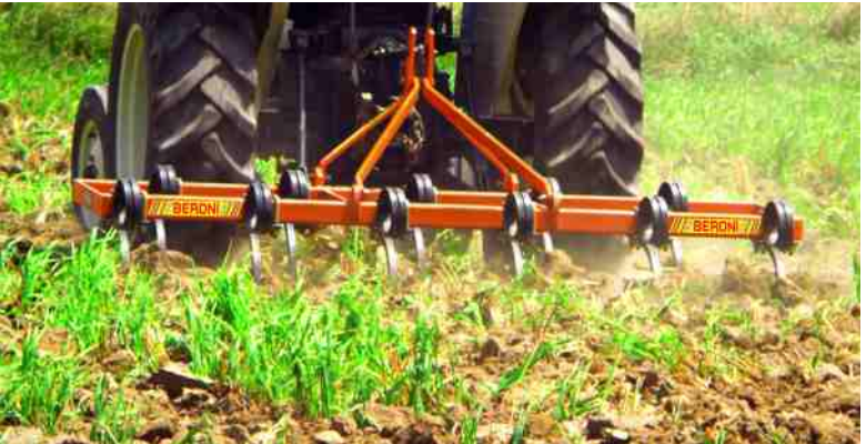
225 mm (9") Double coil tyne of EN-45 material
