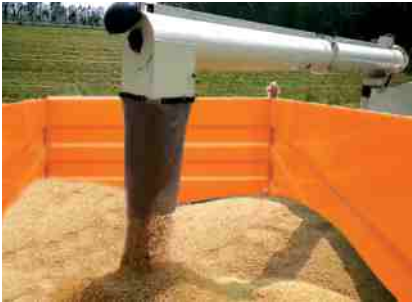
Quick 340° rotating grain discharge auger & hydraulic operated vertical height adjustment
