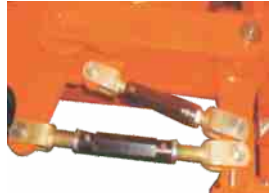
Turn buckle for adjusting of the plough
