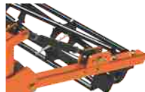
Top link height adjustment of crumbler
